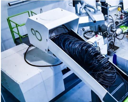
As an all-rounder, the ISEC evo machine processes bulky hose bundles as well as start-up lumps and complete rolls with drip tapes. Photo: PURE LOOP
